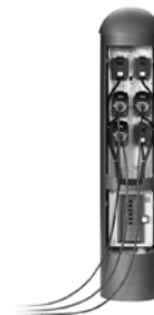
Example of enhanced electrical capacity bollards as manufactured by Hess. The bollards are approximately 48" in height and are customizable, offering up to 8 circuits per box.
