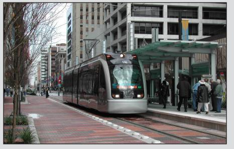
Short passenger rail cars on fixed rails in rightof-way that are separated from other traffic or mixed with traffic, driven electrically from an overhead electric line by an operator on board the vehicle.
