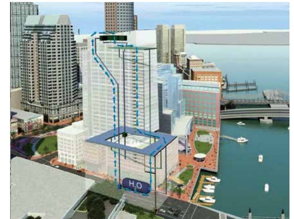
By making use of harvested rainwater, Boston Properties' Atlantic Wharf building is designed to use 15% less water in building HVAC systems compared to a typical building. This illustration shows the flow of harvested water through the building.
