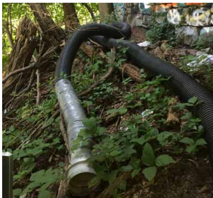
An 8-inch flex hose was observed at the intersection of Hutchinson Avenue and East 5 th Street. This is indicative of septic waste disposal.
