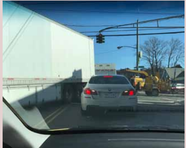
Common situation at many intersections. Streets were not designed to accommodate large semi tractor trailers. Cars at the front of line are forced to back away from the stop bar.
