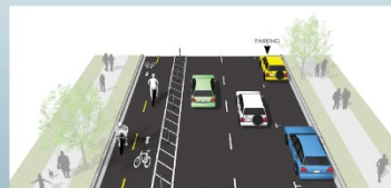
44' Street - Option 4: 2 travel lanes, 1 parking lane, two-way protected bike lane
