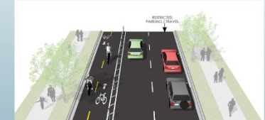
36' Street Option 4: 2 travel lanes, two-way protected bike lane
