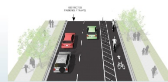
36' Street Option 1: 2 travel/restricted parking lanes, one-way protected bike lane
