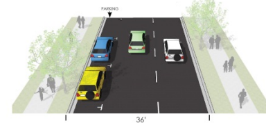
36' Street Existing Conditions: 2 travel lanes, 1 parking lane
