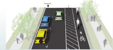
36' Street Option 2: 1 travel lane, 1 parking lane, one-way protected bike lane
