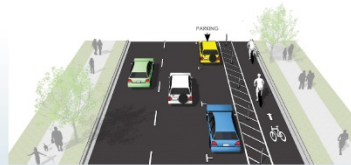
44' Street - Option 2: 2 travel lanes, 1 parking lane, one-way protected bike lane
