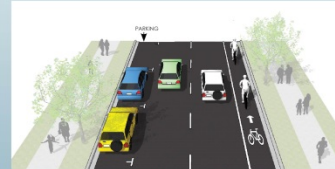
36' Street Option 3: 2 travel lanes, 1 parking lane, one-way bike lane
