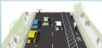
44' Street - Option 3: 3 travel lanes, 1 parking lane, one-way protected bike lane
