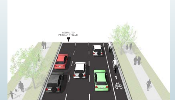
38' Street- Option 4: 2 travel lanes, 1 travel/restricted parking lane, 1 bike lane
