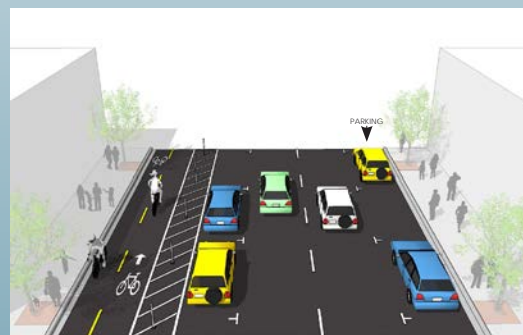
56' Street - Option 4: 2 travel lanes, 2 parking lanes, two-way protected bike lane
