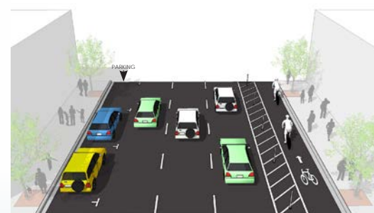
56' Street - Option 2: 3 travel lanes, 1 parking lane, one-way protected bike lane
