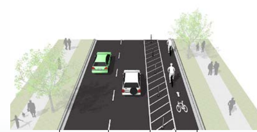
38' Street- Option 1: 2 travel lanes, one-way protected bike lane
