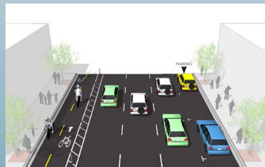
56' Street - Option 4: 3 travel lanes, 1 parking lane, two-way protected bike lane
