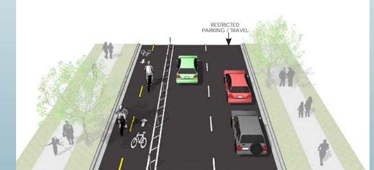
36' Street Option 4: 2 travel lanes, one-way protected bike lane
