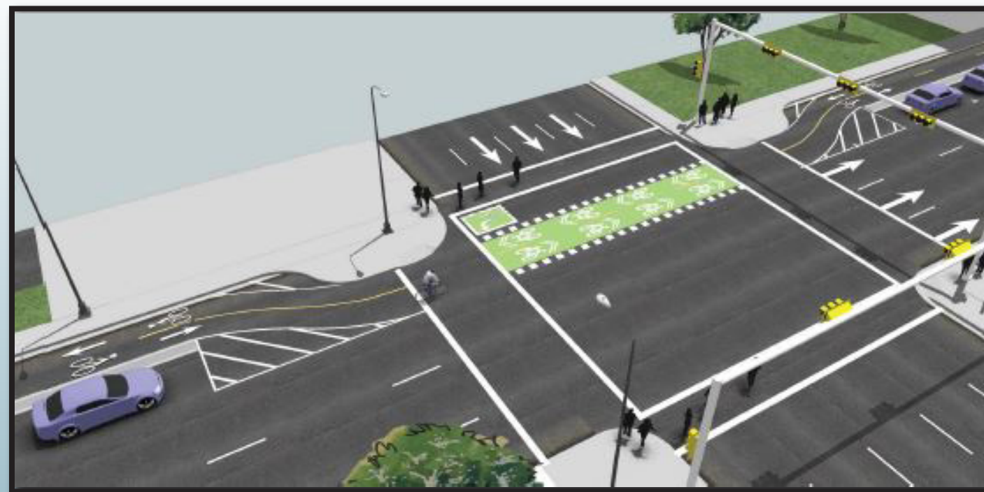
Curb extension incorporated with protected bike lane
