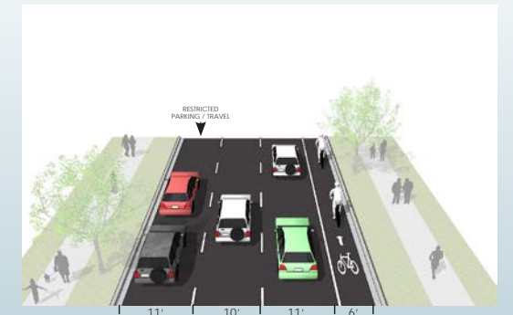
38' Street- Option 4: 2 travel lanes, 1 travel/restricted parking lane, 1 bike lane
