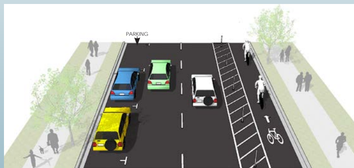
44' Street - Option 3: 2 travel lanes, 1 parking lane, one-way protected bike lane
