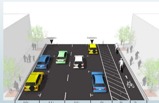
56' Street - Option 3: 2 travel lanes, 2 parking lanes, one-way protected bike lane
