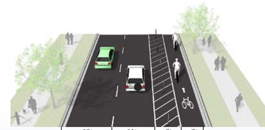
38' Street- Option 1: 2 travel lanes, one-way protected bike lane
