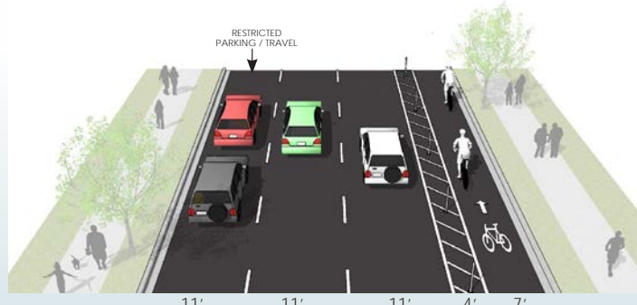
44' Street - Option 1: 1 travel/restricted parking lane, 2 travel lanes, one-way protected bike lane
