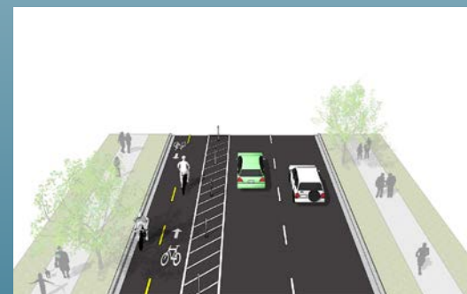
40' Street - Option 4: 2 travel lanes, two-way protected bike lane
